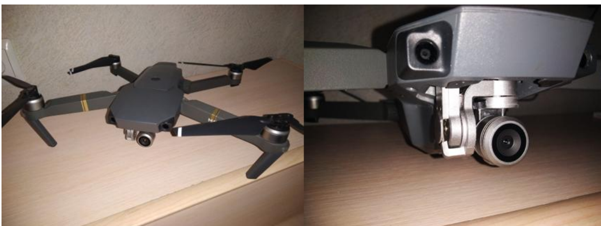
Fig. 4. General view of the UAV and three-axis suspension
