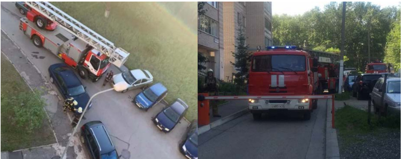
Fig. Examples of obstacles to the movement of fire equipment
