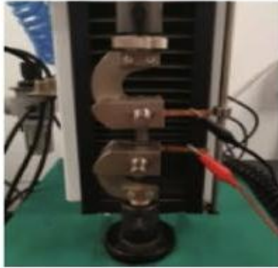
Fig. 12. Installation for measuring the electrical conductivity of a sample during mechanical action on it
