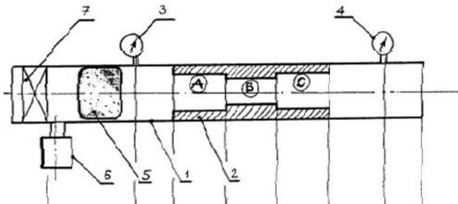
Fig. 1. Scheme for measuring the thickness of ARPD in a pipeline:
