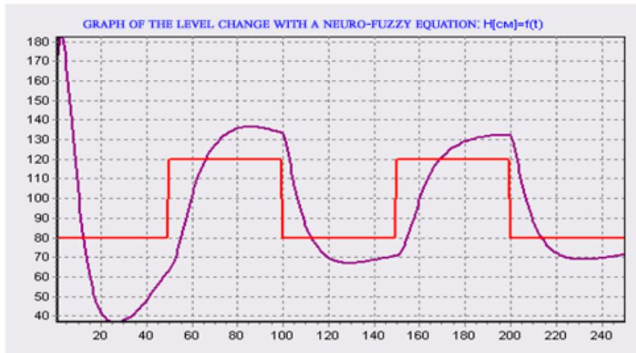
Fig. 7. A transitional process for adaptive neuro-fuzzy control
