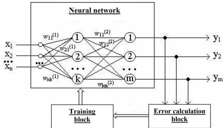
Fig. 1. Neural network with learning and error calculation blocks
