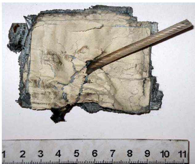
Fig. 1. An improvised device equipped with a piece of fire-conducting cord
