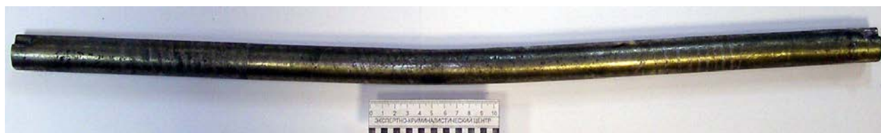
Fig. 3. Metal pipe submitted for examination with traces of the use of a means of transmitting a fire pulse
