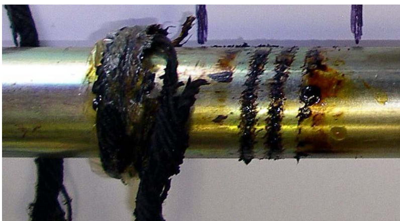
Fig. 4. View of the remains of a burnt-out OSH type fire-conducting cord after a technical study
