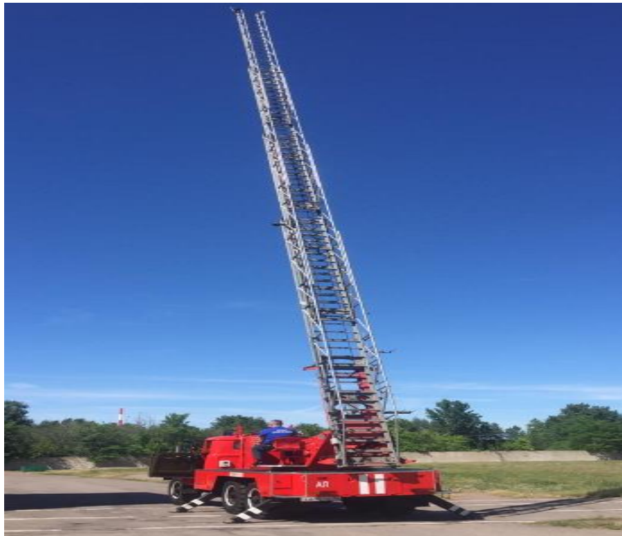
Fig. 3. Extension of the ladder AL-30 (131), not equipped with a removable cradle and the lift was no load
