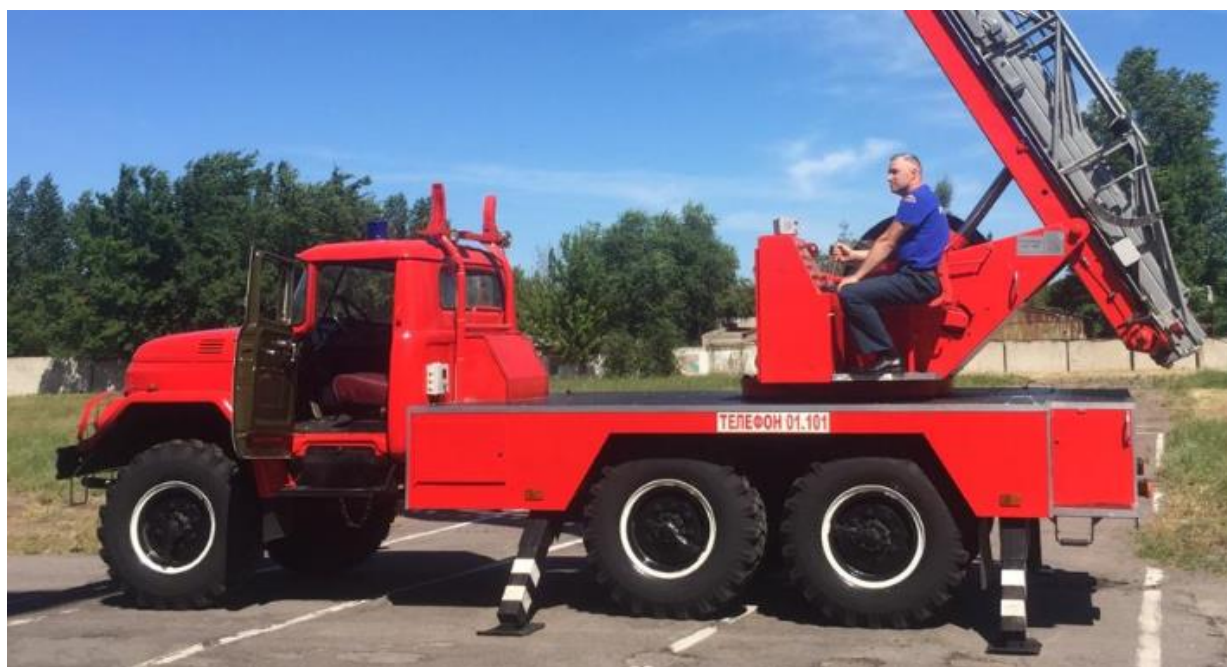
Fig. 2. Extension of the AL-30 (131) supports on a horizontal platform
