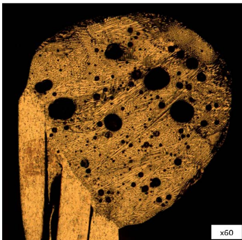
Fig. 5. Panoramic image of the microstructure of the reflow of a sample obtained using a welding machine
