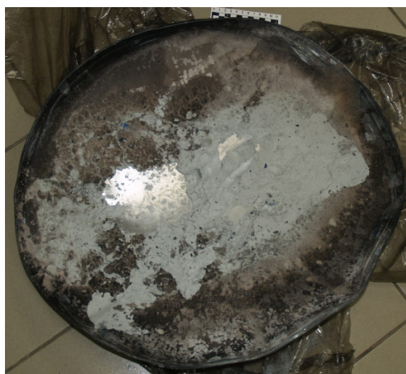
Fig. 2. The lid of a metal barrel received for expertise, with traces of a light gray substance
