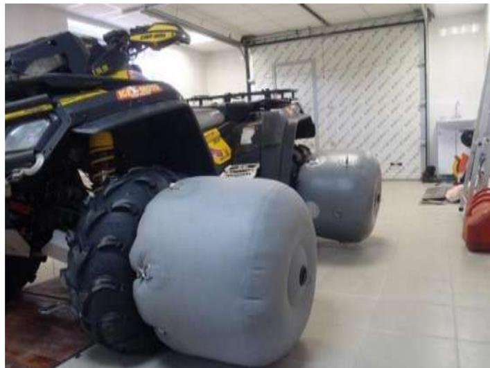
Fig. 5. Inflatable balloon floats
