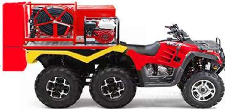
Fig. 4. Layout options of the technical complex by the UPM-300 module with an additional tankage for water
