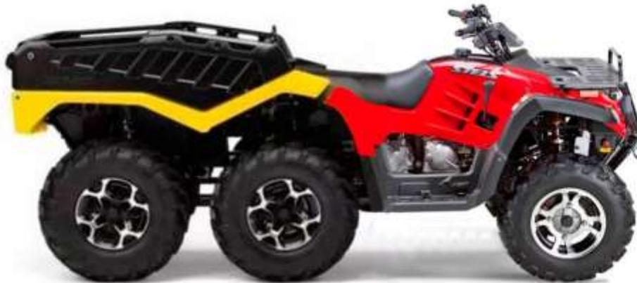
Fig. 2. StelsATV 600 with a module for improving the possibility and carrying capacity
