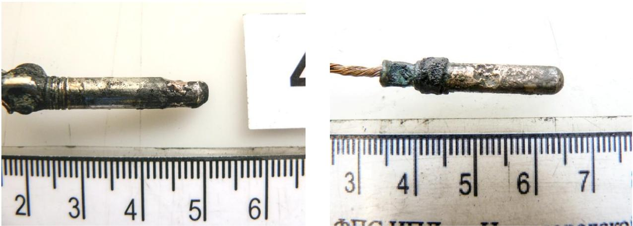
Fig. 3. Destruction of the pins of the plugs as a result of the flow of the spark mode of the LTR
