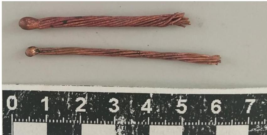
Fig. 2. Reflow copper conductors selected for XPhF
