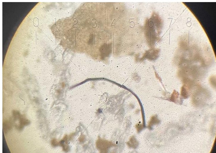
Fig. 15. Sample № 3. Black fibrous microplastic
