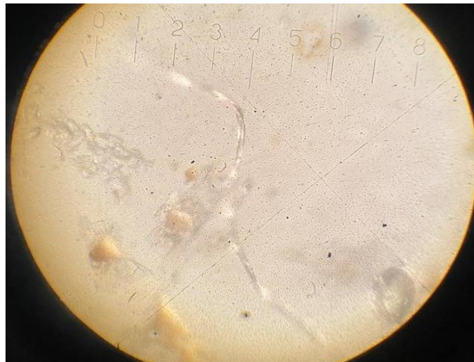
Fig. 6. Sample № 6. Microplastic transparent fibrous form
