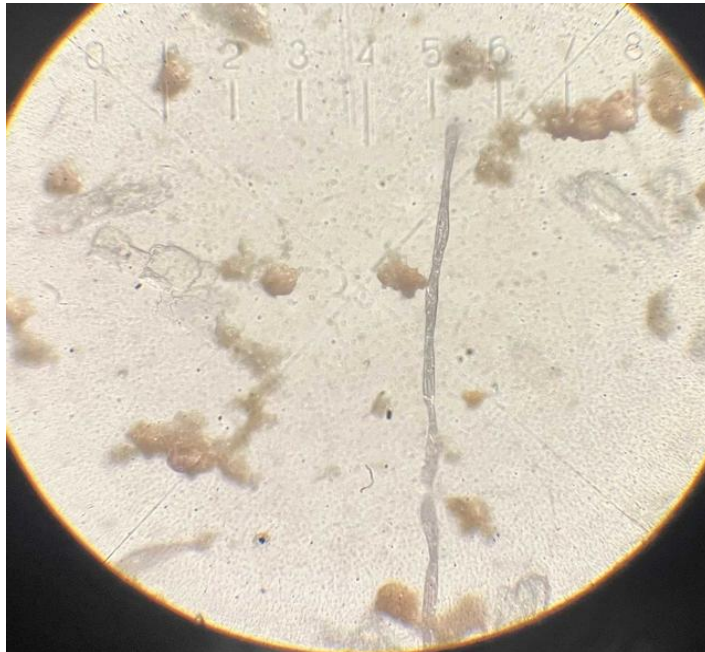
Fig. 12. Sample № 3. Microplastic transparent fibrous form
