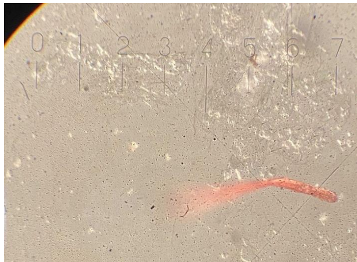
Fig. 7. Sample № 6. Red fibrous microplastic
