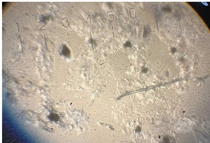
Fig. 1. Sample № 7. Microplastic fibrous form of a transparent color
