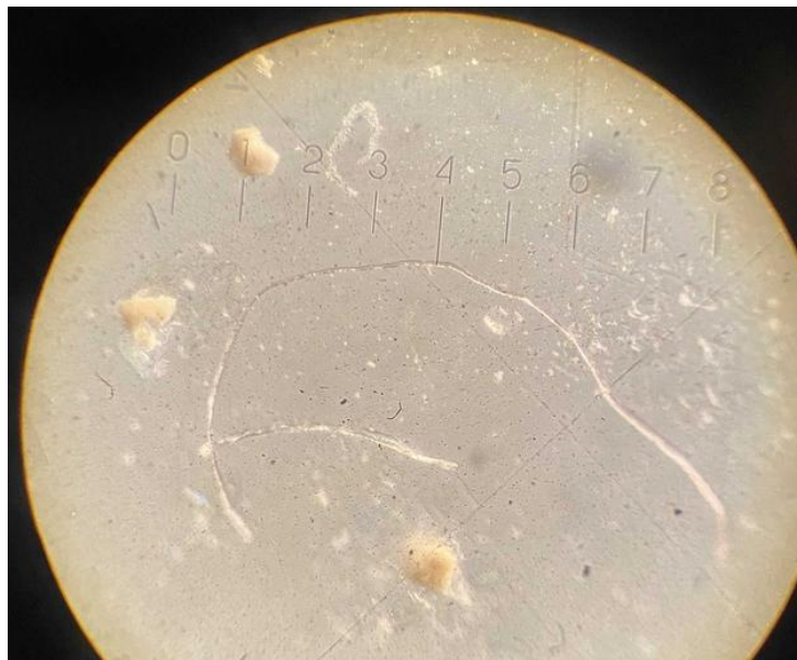
Fig. 3. Sample № 7. Microplastic fibrous form of a transparent color
