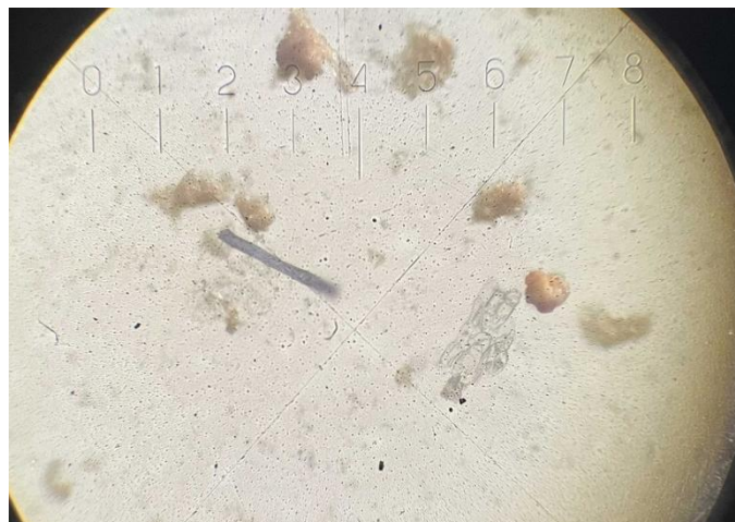
Fig. 10. Sample № 4. Microplastic transparent fibrous form
